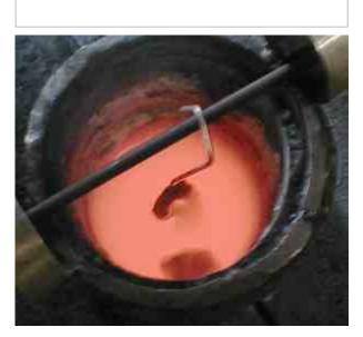
pot appears to be full of a translucent orange fluid and as the blade slips under the surface, you can see the color move into the blade. Eventually (in about 30 seconds), there is a dark shadow in board of the spine and then even that winks out. Let it soak for maybe another 30 seconds and remove it.
