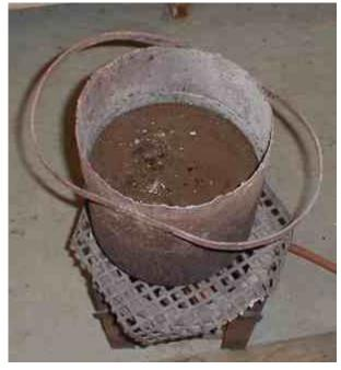
It is poured (carefully!) into the pot. The element is attached to a <u>variac</u> and powered up. I then watch to see that the temp is increasing. If it is, all is good. If it isn't, I can bail out by pouring the salt back into the kettle or jumping to turn-off procedure, and then swap out the element. Trust me - getting congealed salt out of a pot with a blown element is NO fun.
