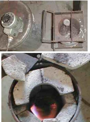
after lighting off. At 8..10 psi, the temp rise is approximately 5 F/minute. Given the mass of the tube, I've elected to run the temp up slowly and not overshoot. While the pot is humming to itself, the time is
